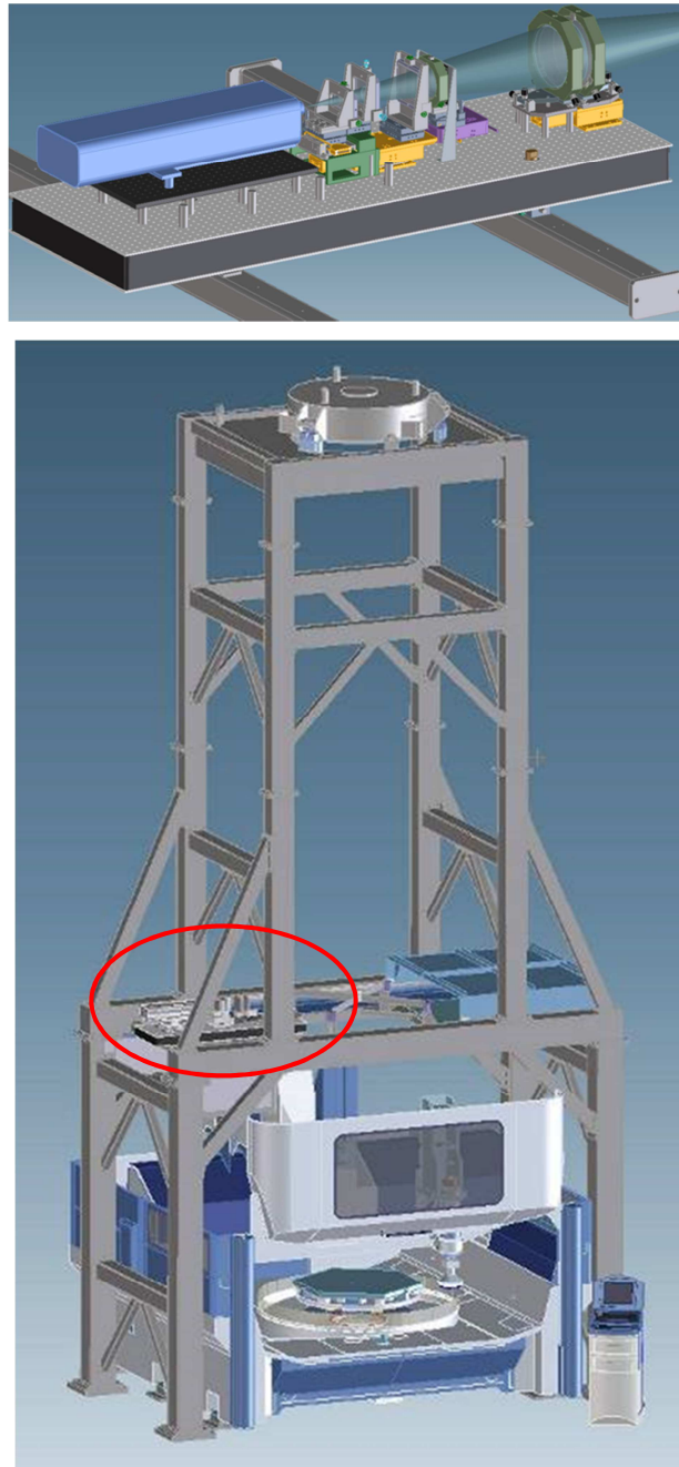
Figure 2. A schematic of the Glyndŵr University E-ELT prototype segment optical test. The top figure is a detail of the optical breadboard on which the refractive optics are integrated. A spider assembly and small fold mirror diverts the beam emanating from the breadboard to the top sphere at the top of the test tower and then to the optic under test on the polishing machine. The top sphere is instrumental in reducing the optical path length of the test from a nominal 160 m to approximately 32 m.
