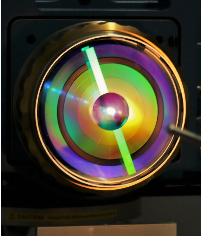
8 zone CGH for the alignment of the Euclid space telescope
