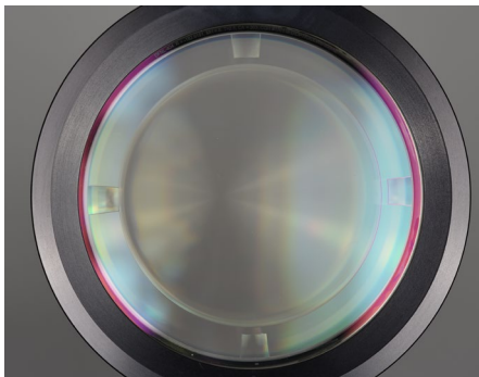
DFNL with adjustment hologram
